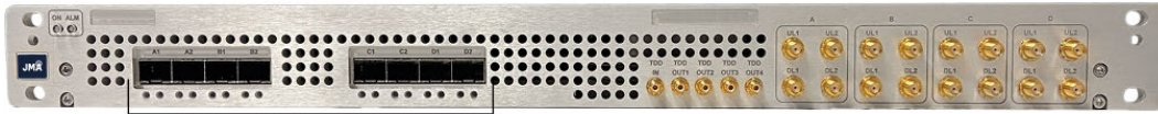
A1 A2 B1 B2 C1 C2 D1 D2 Optical ports for connection to next generation remote units
