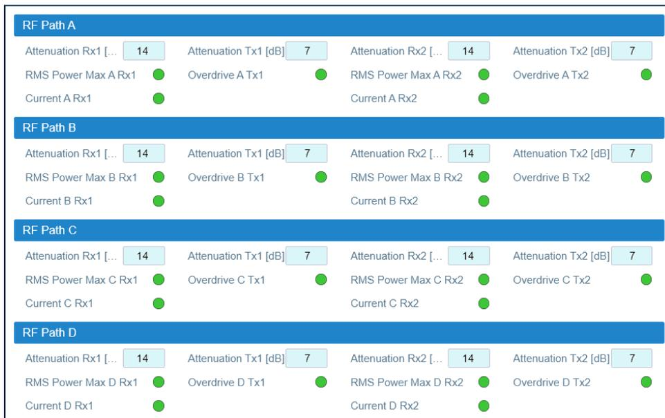
2. To increase the downlink RF gain for a specific RF path, reduce the *Attenuation Rx1* and *Attenuation Rx2* in the appropriate **RF Path** pane (RF Path A, RF Path B, RF Path C, RF Path D).
